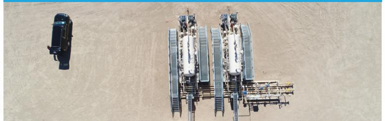
Our Delaware Basin team is developing a robust infrastructure that supports oil, water and natural gas gathering. Our tankless facilities only a separator and pumps to gather product from the wellhead and transport it into a gathering system, removing the need for multiple separators, tanks and flares.
